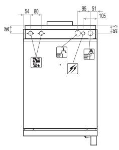
Overall dimensions (W x D x H) - mm
