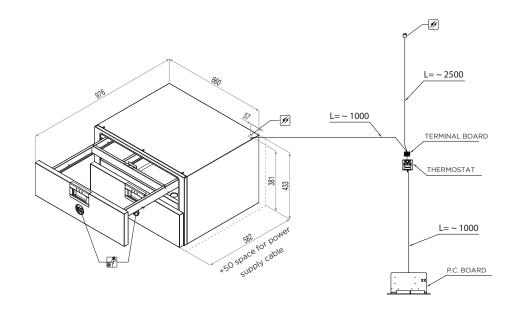
Overall dimensions (W x D x H) - mm
